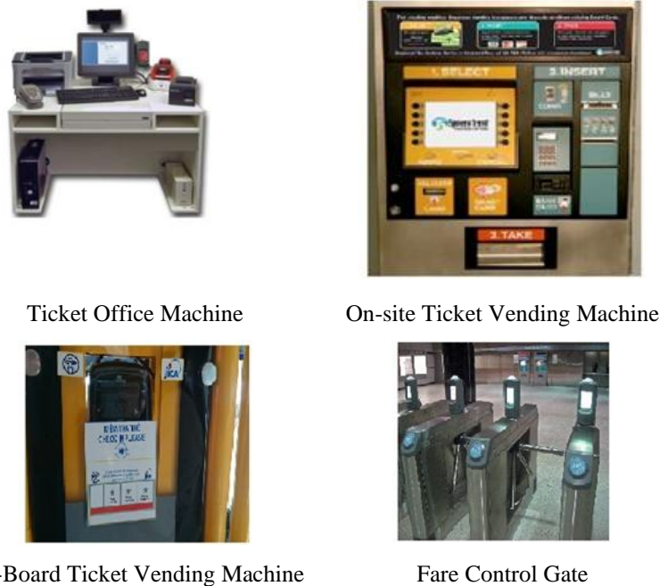
Figure 3. Devices to Read/Write Fare Media [6].
