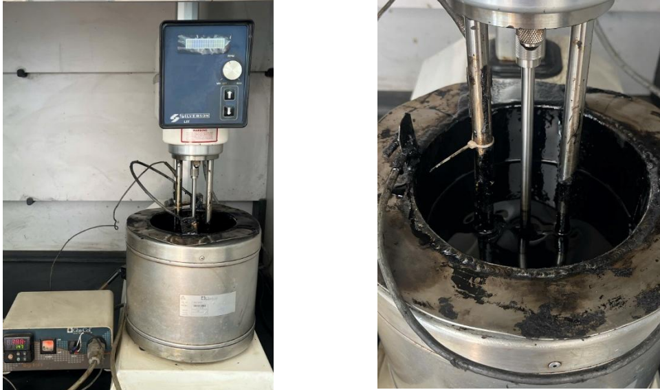
Figure 2. Equipment for mixing TPS additive into 60/70 asphalt binder.
