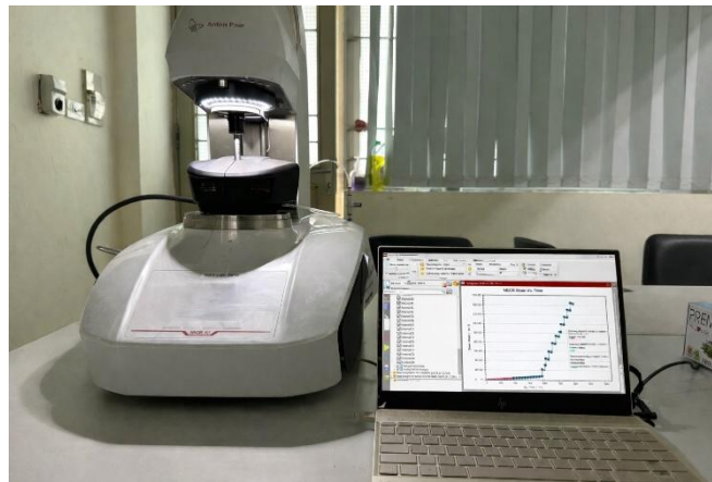
Figure 4. Dynamic Shear Rheometer (DSR) manufactured by Anton Paar.
