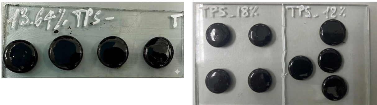
Figure 3. Modified asphalt binder samples prepared with TPS additive.
