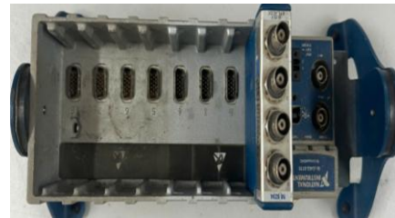
b) Data acquisition unit NI cDAQ-9178 + Module NI-9234.
