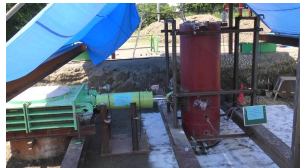
Figure 2. Experimental setup and lateral loading arrangement (Photo taken by research group).
