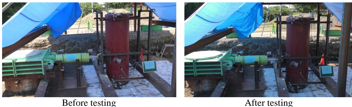
Figure 5. Pile condition before testing and deformation profile after the lateral loading test (Photo taken by research group).
