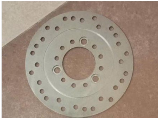
a) Standard brake disc model of the Honda Lead (SCR)
