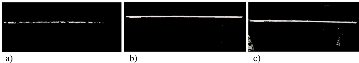
Figure 10. Sensitive investigation on the tolerance of the LCS algorithm: a) tolerance of 5; b) tolerance of 50; tolerance of 100.
