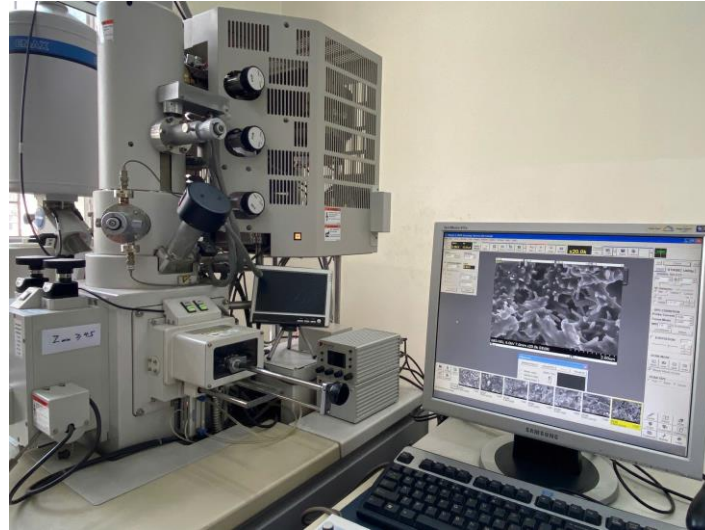
Figure 7. Microstructural analysis of cement-asphalt emulsion asphalt samples.
