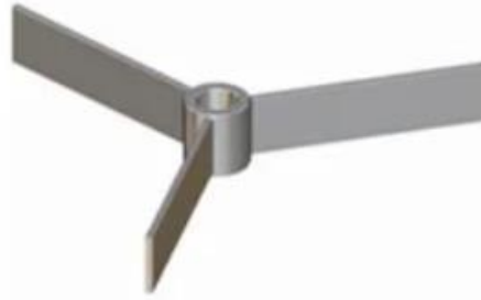
Figure 1. An example of the flat-blade turbine can be fabricated by both the ‘WAAM + CNC machining’ and ‘CNC machining’ approaches.
