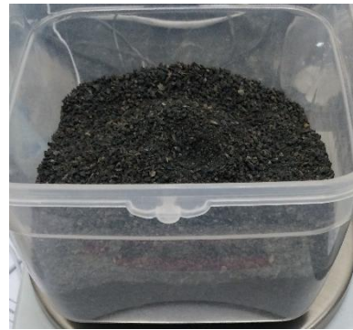
Figure 4. Crushed LWS from lava stone waste.
