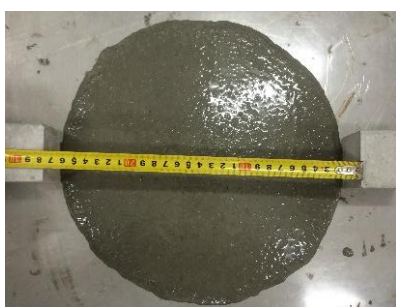
Figure 6. Flow of mortar.
