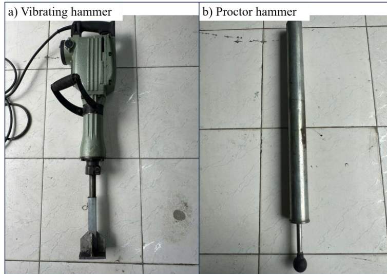
Figure 7. a) A vibrating hammer, and b) A Proctor hammer.
