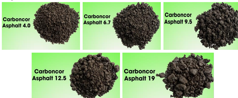
Figure 1. Classification of carboncor asphalt materials (figures provided by Carboncor Vietnam).
