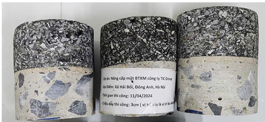
Figure 9. In-situ samples to perform direct shear test.
