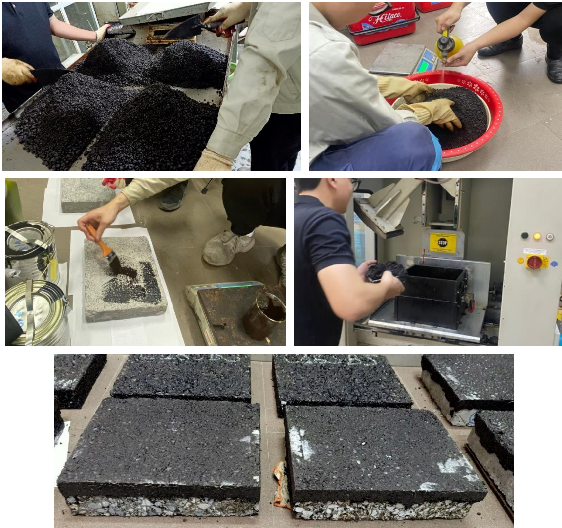
Figure 7. Steps for preparation of testing samples.
