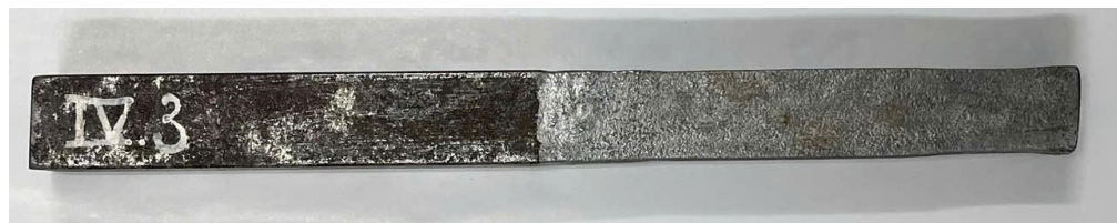
Figure 3. Morphology of steel samples after 240 hours of corrosion.
