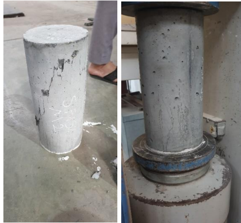
Figure 2. Test of compressible strength in SF15 specimen at 3 days of age.
