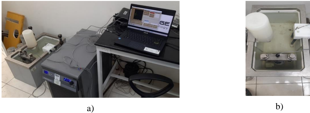
Figure 3. Thermal expansion coefficient measuring device: a) general view of device; b) Sample immersion tank for measurement.
