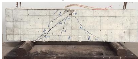
Figure 12. Failure pattern on specimen OSCB-S-50 with 50% natural sand volume replaced by crushed oyster shells.
