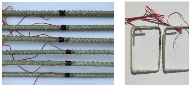
Figure 5. Strain gauges are glued on the face of GFRP reinforcement.
