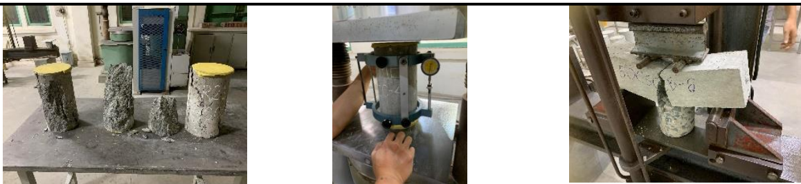
a) Compressive strength test b) Modulus of elasticity test c) Tensile flexural strength test
