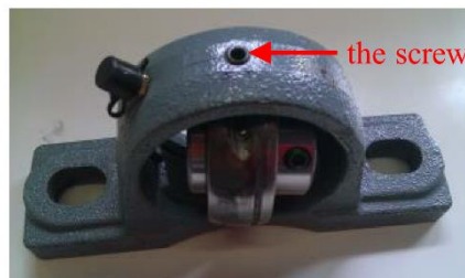
Figure 8. Bearing with artificial outer raceway defect.
