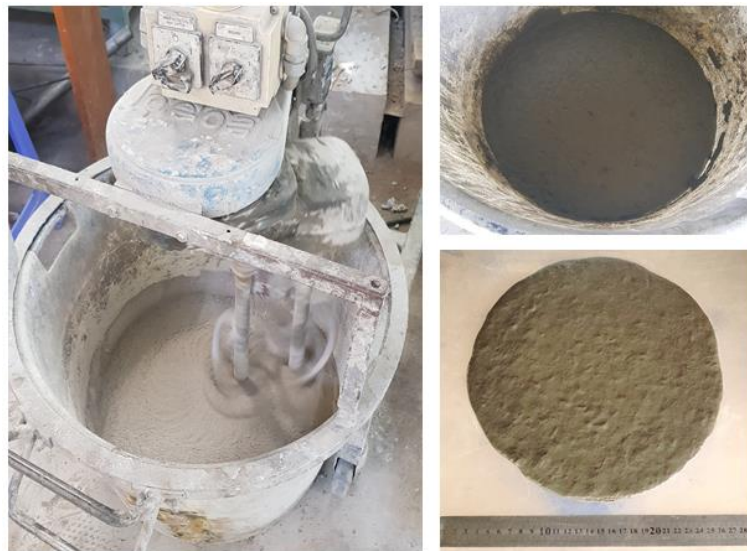
Figure 3. Laboratory mortar mixer (left) & freshly mixed HPFRM mixture (right)
